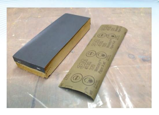
The wet sanding process begins with 320g paper. An easy D.I.Y. system uses a standard sheet of sandpaper cut to fit a 9.5" sanding block and stapled in place. The 320g finish can be followed by 400g, 600g or even finer depending the finish desired.
