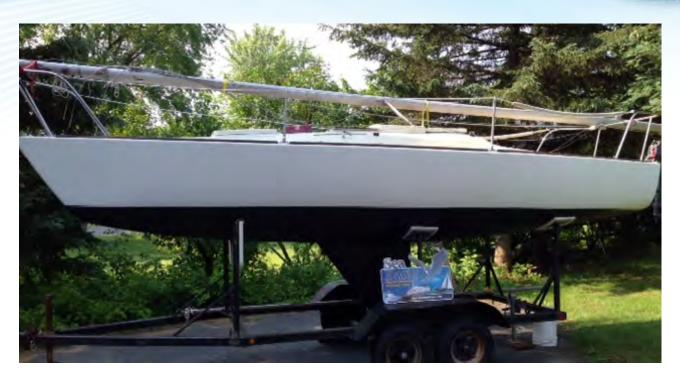
This is a freshly sprayed Biocop TF black bottom. About 50% more paint was applied than normal in anticipation of a wet sanded racing finish. Allow the paint to cure for about a week prior to burnishing the finish.
