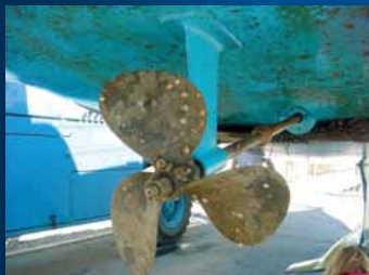
Smart Solution on sailboat after one season. Hard growth on non-painted running gear; none on the hull.
